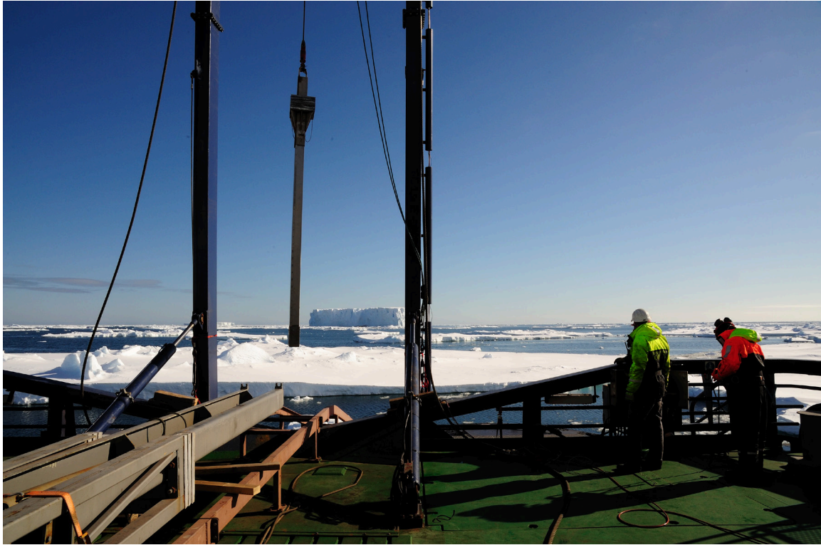
The 3 m long Kasten corer lowered into the water using the A-frame of the Oden.
