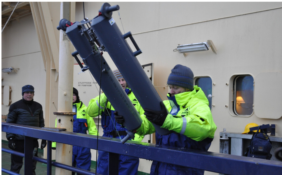
Niskin sampler deployed from the starboard side of Oden
