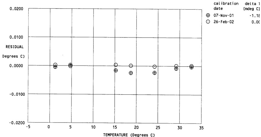
**Underway Remote Temperature Sensor (Wet Lab)**
