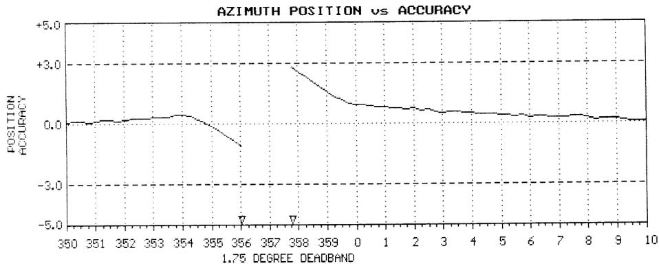
NOTE: Azimuth Position vs Accuracy graphs are accurate to within 0.5 degrees. The accuracy shown in the potentiometer deadband region between 355 and 0 degrees is the result of no resistance change while position changes. The gap represents the actual deadband (open circuit).
