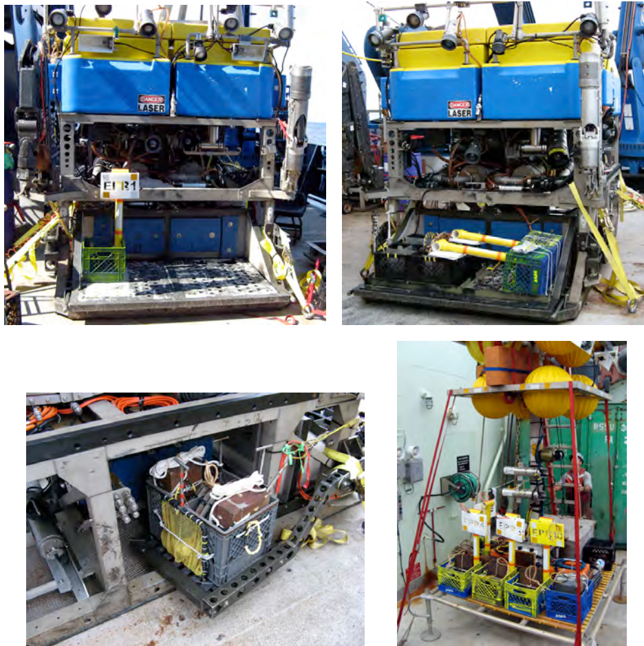
Figure 4b-1. Photos of JasonII and elevator prior to Dive 268. Upper left photo shows benchmark design, upper-right photo shows arrangement of Benchmarks 1&2 on basket along with sample basket prior to launch. Lower left shows syntactic float packs rigged on swing arms. The float packs were attached to the OBSs to provide additional buoyancy. Lower right photo shows elevator rigged with additional benchmarks (foreground) and sample basket in wooden box (background).
