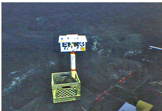
Figure 4.b-4. A) Dimensions of EPR ISS Benchmarks. B) Digital photographs taken from JasonII of the four EPR ISS Benchmarks installed during Dive 268.
