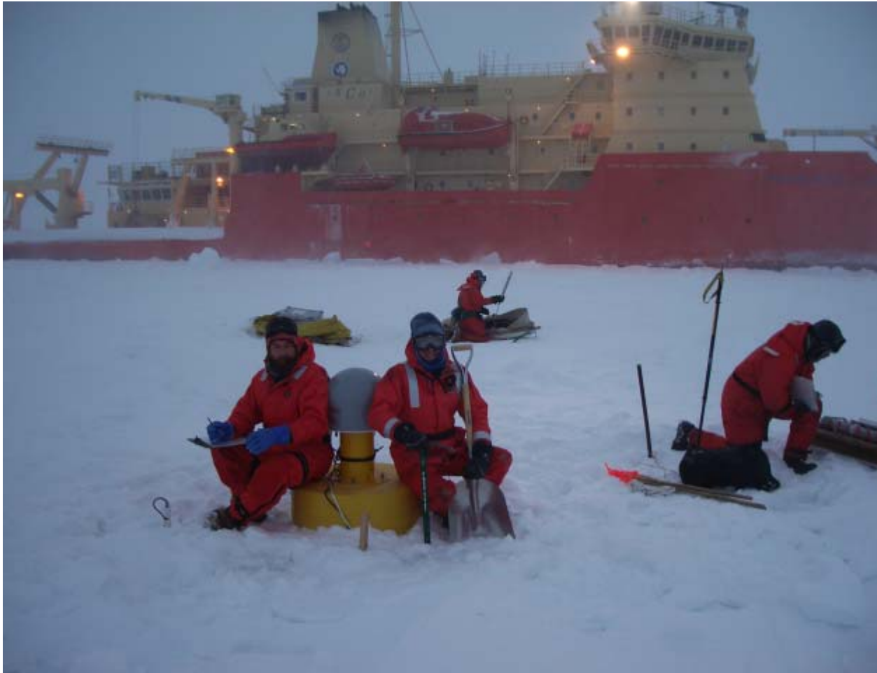
Figure 5. Flux buoy deployment during the Phase 1 survey. The radome shelters the GPS and iridium modem antennas, and the top of the thermistor string can be seen in the lower left of the photograph. The temperature/conductivity sensor is suspended 8m below the buoy within the ocean mixed layer.
