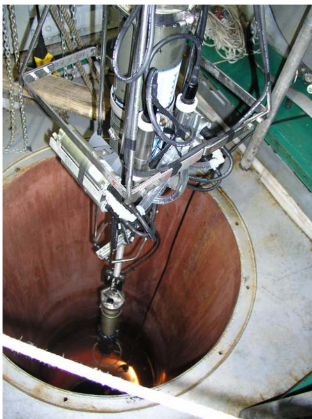
Figure 1. A photograph of the CTD profiler (upper instrument) and microstructure instrument (lower) hanging over the moon pool just prior to deployment. The microstructure sensors were at the bottom of the suspended package 1.5m lower than the CTD package. These instruments were continuously raised and lowered through the water column at 0.6 m/s between 18m and 350m depth by a computer-controlled winch.
