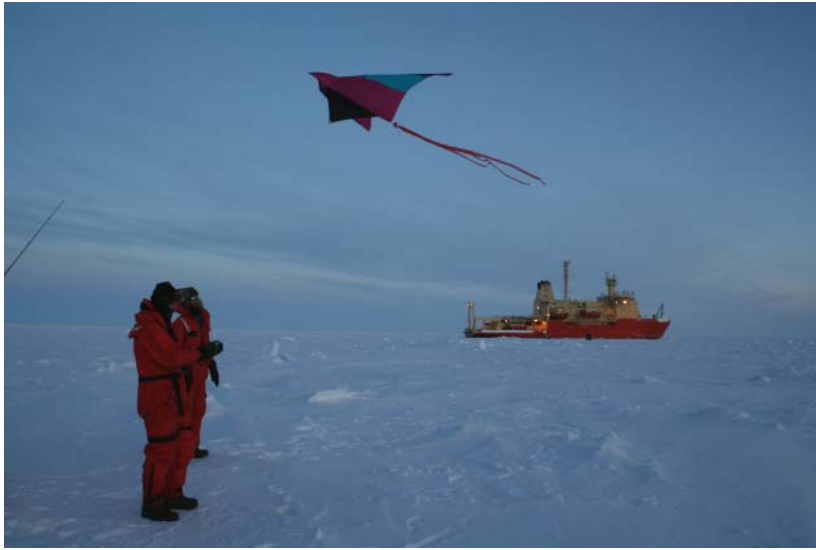
Figure 7. Preparing to launch rawinsonde instrument package beneath a kite for studies of downwind effects of a lead (20 m to the left of the scene), during Phase 2, Drift 2. [deSteuer photo]
