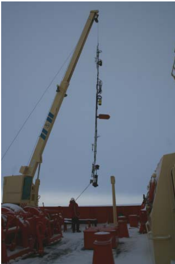
Figure 4. The deep mast assembly being hoisted into position with the forward crane (left). Between deployments it was stowed in two sections suspended beneath the forward cargo hatch. For Phase 2 operation, it was deployed through a hydrohole near the bow, shown here during the recovery of P2D2, after cracks had appeared off the bow (below). [Stanton, deSteur]
