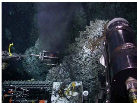
Figure 2.13.3. Rotary flow meter measurement at Stonehenge vent.
