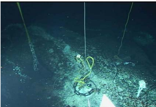
Figure 2.6.5. Final RAS setup for 2008-9, which is nearly identical to the 2007-8 setup. The intake is very near the edge of the crack under the vent cover. An MTR to be recovered next year is in the lower right of the photo, and an abandoned osmosampler is across the crack.
