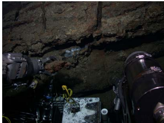
Figure 2.13.2. Sampling of an extinct sulfide from the 'log' on the west side of the Faulty Towers complex.
