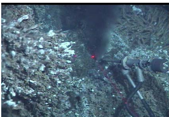
Figure 2.12.3. High-temperature fluid sampling at Hulk vent.
