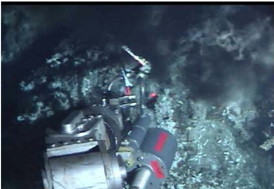
Figure 2.11.3. Red major fluid sample collected in 331°C fluid a few meters from the RAS site.
