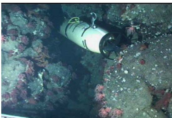
Figure 2.14.6. The AUV lodged in a crevice in a near vertical scarp along the side of Summit Seamount.
