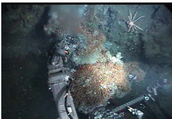
Figure 2.9.5. High temperature fluid sampling at Puffer vent.
