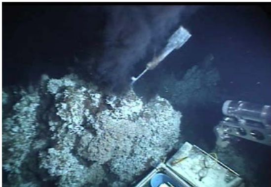
Figure 2.2.1. Hobo temperature probe retrieval from Dante vent.
