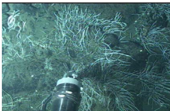
Figure 2.9.4. Fluid sampling at a diffuse vent at Easter Island where the RAS sampler was deployed in 2007-8.
