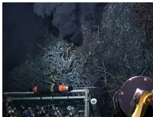
Figure 2.16.2. High-temperature fluid sampling at Boardwalk vent.
