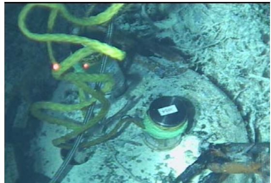
Figure 2.6.4. Vent cover for the newly deployed RAS at Marker 33. Temperature recorders 3054 and 3087 are placed in the cover and 3173 is attached to the intake line under the cover.
