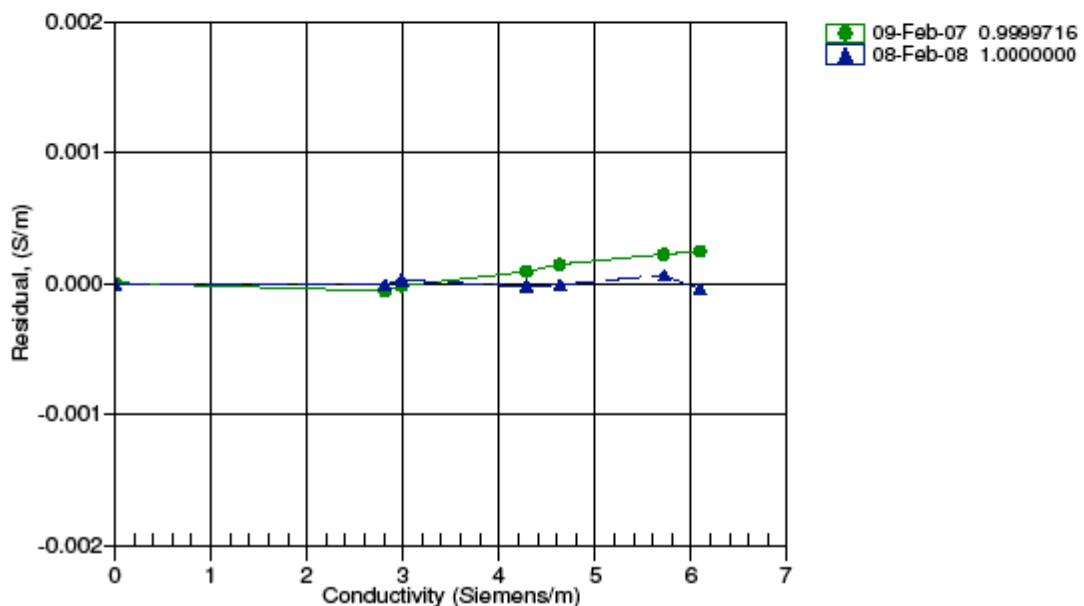
**Secondary Conductivity Sensor****SEA-BIRD ELECTRONICS, INC.**
