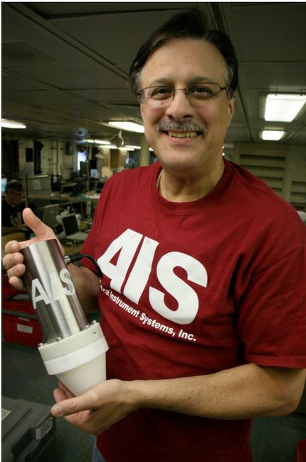
Figure showing transceiver size. The white part is the antenna section. The titanium part holds the electronics and could easily hold a battery pack for future instrument data collection.
