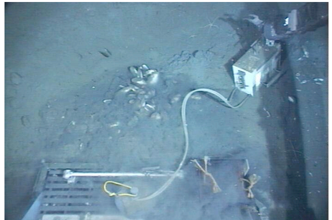
Left image: Hydronode with sensor probes stretching out to the right. Right image: Flow chamber, resistivity and heat flow probes placed in seep site
