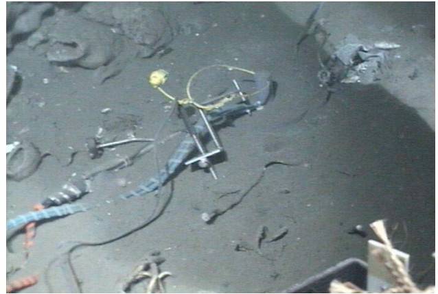
Left image: Hydronode with sensor probes stretching out to the right. Right image: Flow chamber, resistivity and heat flow probes placed in seep site
