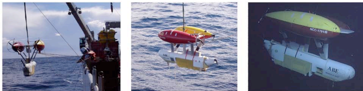
Figure 4. Left and middle image show ABE being launched while JASON2 was operating on the seafloor. Right image shows ABE entangled in an old mooring line ~100 m above the axial valley floor. The line was cut using JASON 2 and was brought back onboard safely.
