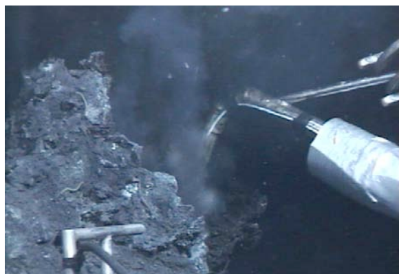
Figure 11. Hot Harold deployment of the sensor housing
