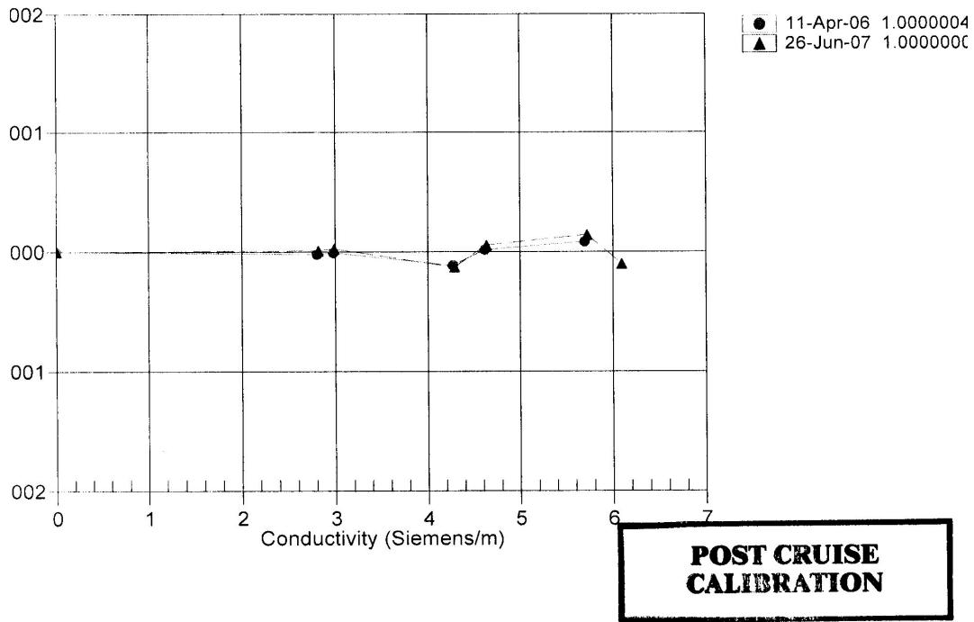
***CTD Secondary Conductivity Sensor (cast 007 – on)***
