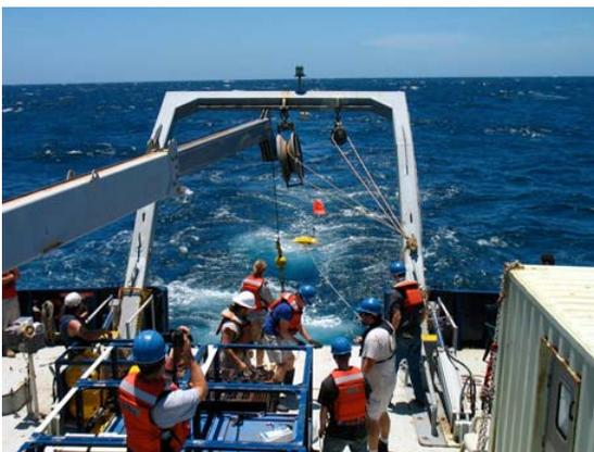
Deploying the float and data logger package off the stern using the crane under the A-frame.
