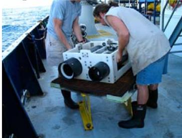
Place the acoustic and data logger frame on the anchor and attach the release to the frame.
