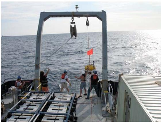
Retrieving the first part of the tethered instrument using the A-frame.
