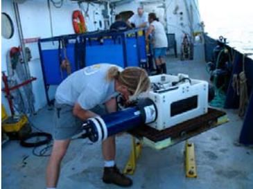
After programming the data logger in the science lab, place it inside the frame and secure it.
