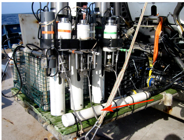
Figure 13. Photograph of Alvin 's basket as configured for this cruise showing placement of the magnetometer (red arrow pointing to long white tube laying on the basket), and Seewald gas-tight water samplers (vertical cylinders with colored tape).
