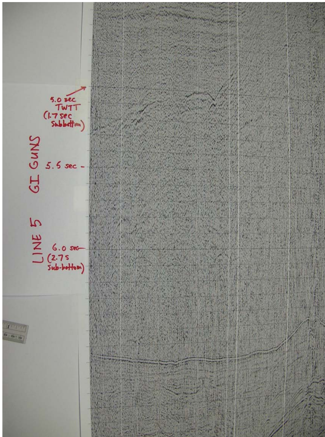
Figure 4. Photograph of a portion of seismic line NZ-5, showing the same survey area as in figure 4.3, but shot in the opposite direction (E to W). The reflector at 5.3-5.5 sec is the top of the volcanic basement. Thin black lines are at 0.1 sec intervals of TWTT. Note distortion of the right side of the photo.
