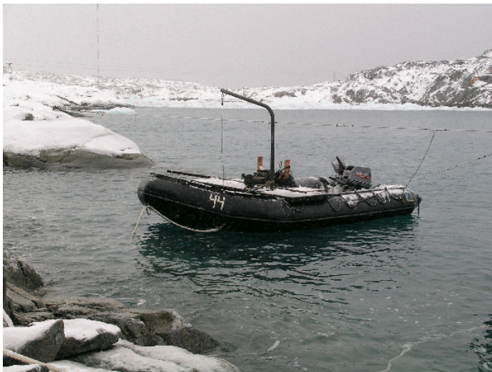
3 Zodiac #44 showing the platform and davit that were used for the towed sidescan, Seacat, and video camera work.
