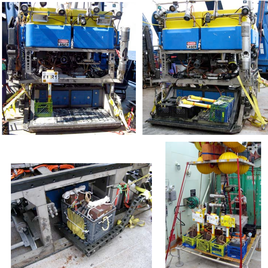
Figure A. Photos of Jason2 and elevator prior to Dive 268. Upper left photo shows benchmark design, upper-right photo shows arrangement of Benchmarks 1&2 on basket along with sample basket prior to launch. Lower left shows syntactic float packs rigged on swing arms. The float packs were attached to the OBSs to provide additional buoyancy. Lower right photo shows elevator rigged with additional benchmarks (foreground) and sample basket in wooden box (background).
