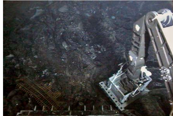
OBS206 anchor buried in lava - after release
