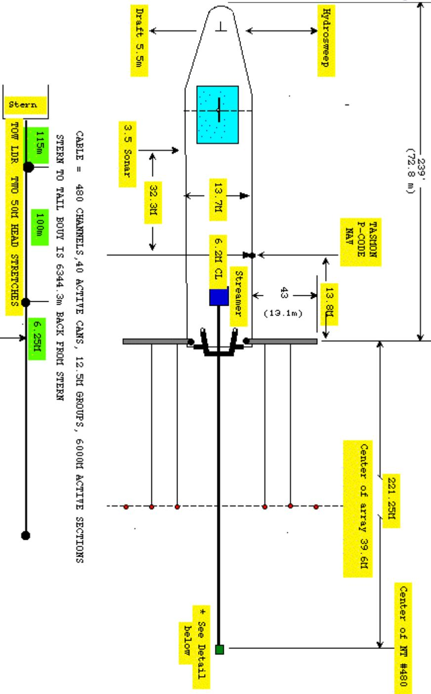
12 AIR GUN ARRAY DETAILS 6MT STREAMER
