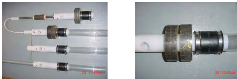
Figure 29. Detailed images of the gravity corer used (source: http://www.aquaticresearch.com ).
