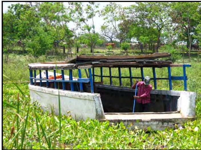
Figure 8. The Morrino No. 2 was unloaded from a semi-truck into the mud flats of the Tipitapa River mouth in Lake Managua. This boat could maneuver shallow waters and mud flats powered by a 40-horse-power outboard motor. The dock consisted of two long planks set up on blocks. (Photo by Steffen Saustrup)
