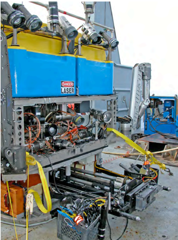
Front of Jason2 ROV showing drill system barrels and 'points' used to anchor the ROV to the seafloor outcrop/structure during drilling. Baskets on either side are holding instruments to be deployed in drilled holes and fluid samplers.
