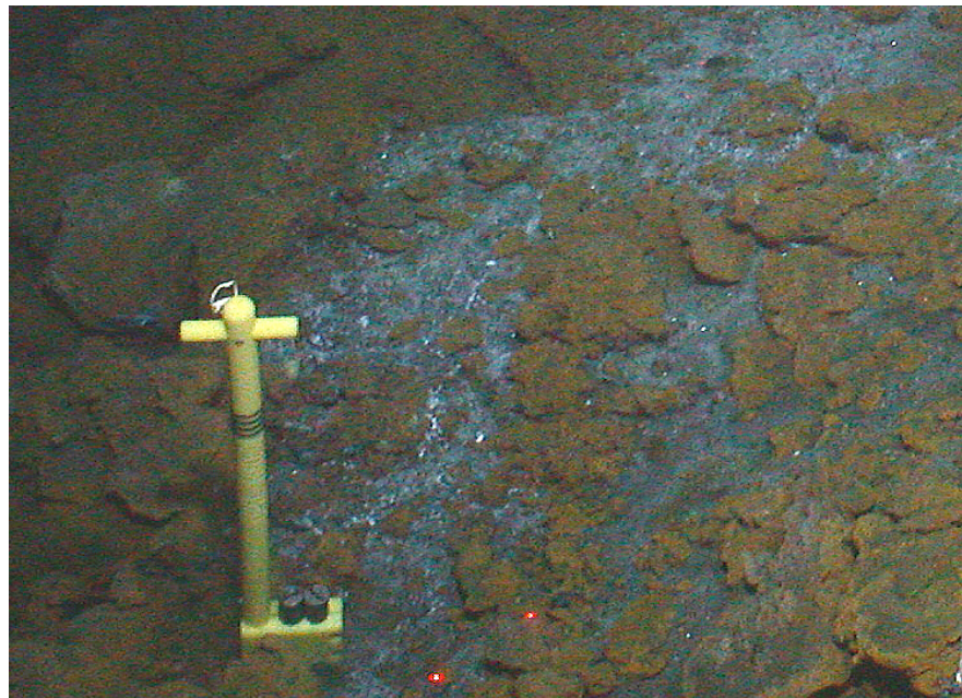
Figure 8. Example of low-temperature probe wand deployed in fissure venting shimmering water. The yellow wand holds two of the VEMCO probes at its base, which penetrate through the sediment veneer on the surface of the fissure. The top of the wand has a T-handle for ease of handling with Alvin or Jason2 manipulators.
