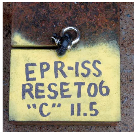
Photographs of transponder anchors used at EPR ISS during AT15-06. Note pull-pin arrangement, designed so that transponders can be recovered after ~ 3 years and re-battered and redeployed.
