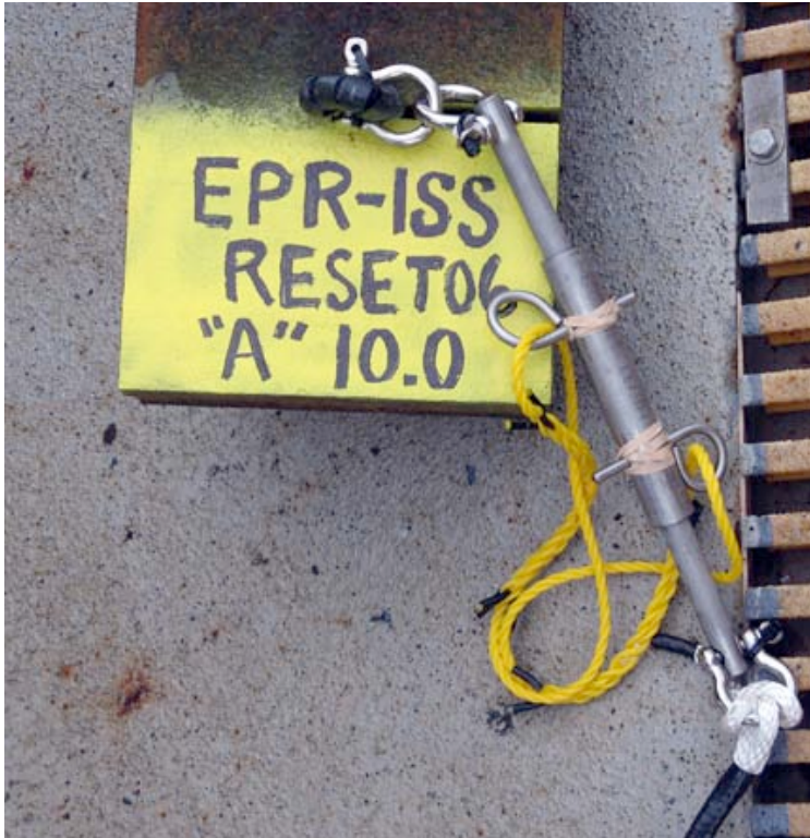
Photographs of transponder anchors used at EPR ISS during AT15-06. Note pull-pin arrangement, designed so that transponders can be recovered after ~ 3 years and re-battered and redeployed.
