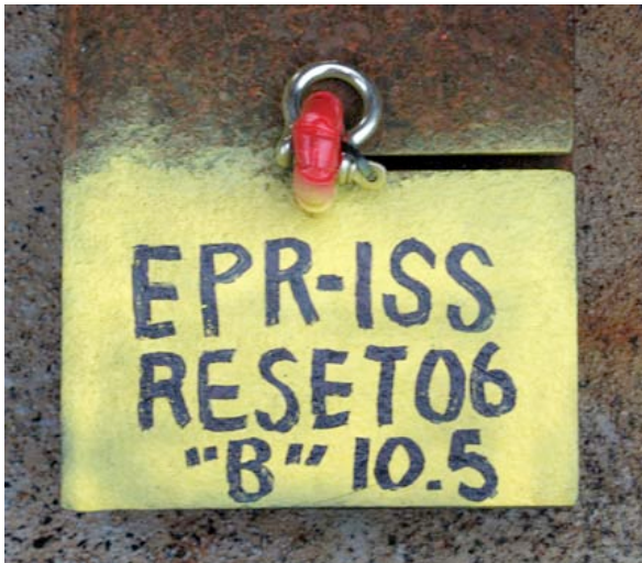
Photographs of transponder anchors used at EPR ISS during AT15-06. Note pull-pin arrangement, designed so that transponders can be recovered after ~ 3 years and re-battered and redeployed.
