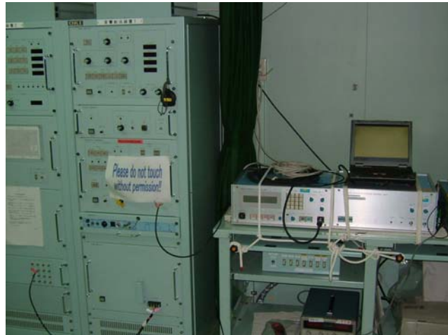
Photo 4-4-2. Main unit of “Kairei” SSBL (left), and acoustic on board units of JAMSTEC (middle) and of Kobe Univ. (right).
