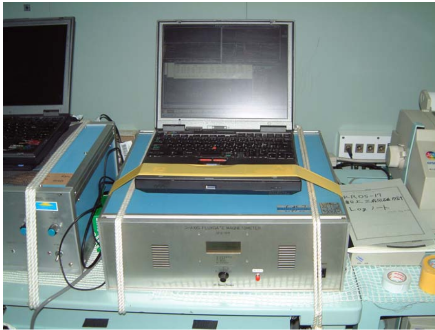
Photo 4-6-3. Magnetometer control unit and data logger. Geocentric coordinate geomagnetic intensity can be seen on the PC display.
